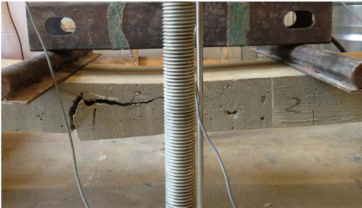
Figure 7: Image of Four-Point Load Testing for Panel P-4
