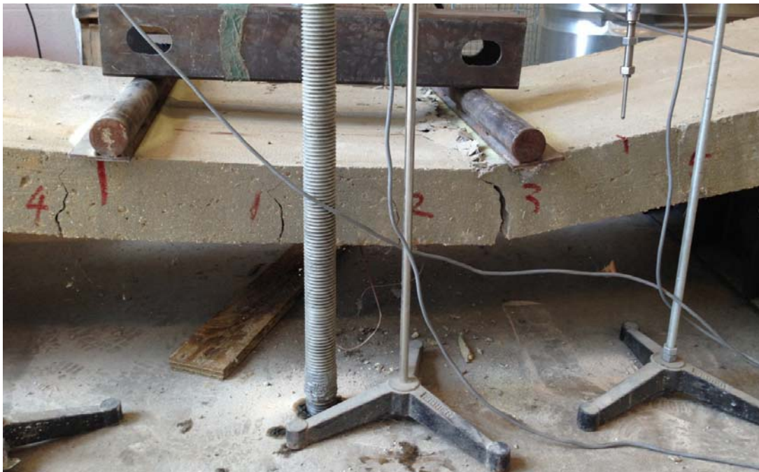
Figure 5: Image of Four-Point Load Testing for Panel P-2
