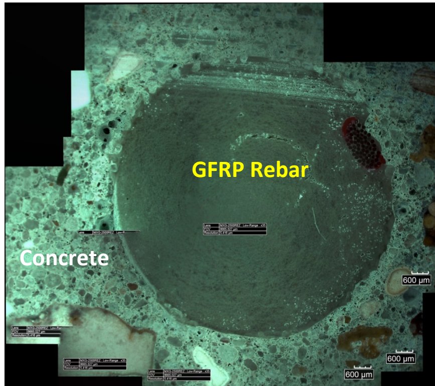
Figure 14: Microscopic image for sample from Panel P-5
