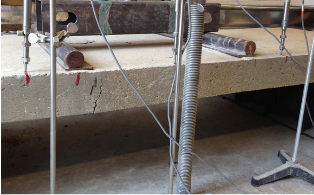
Figure 6: Image of Four-Point Load Testing for Panel P-3
