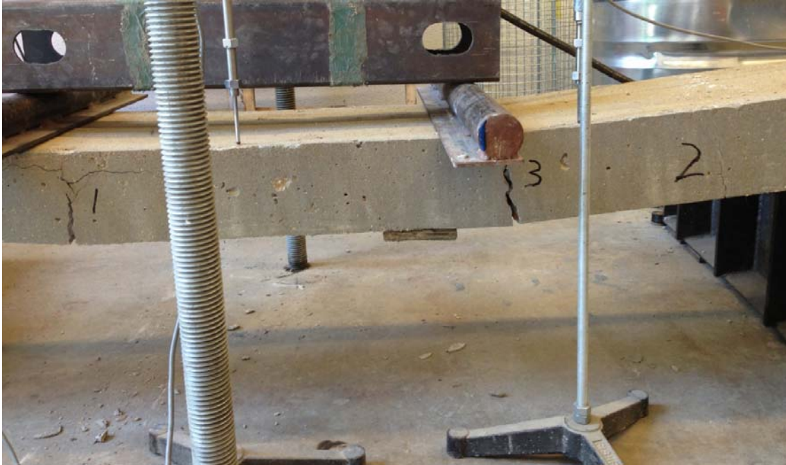
Figure 8: Image of Four-Point Load Testing for Panel P-5
