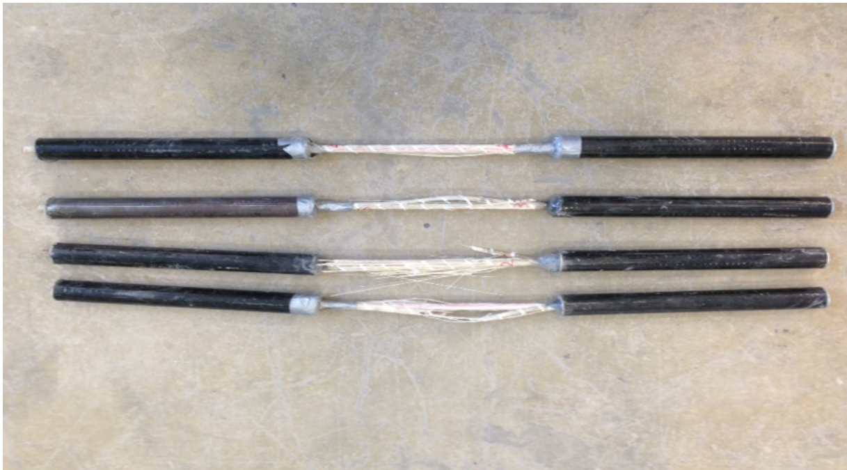
Figure 3: Post Test: Fractured GFRP bar specimens
