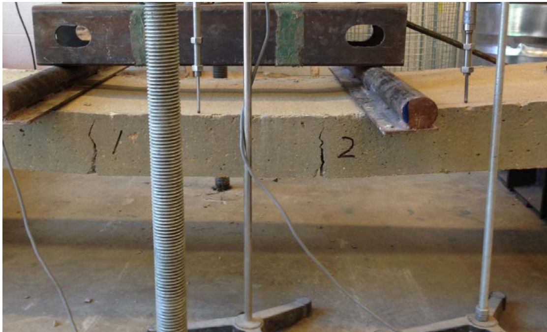
Figure 9: Image of Four-Point Load Testing for Panel P-6
