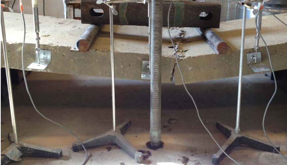
Figure 4: Image of Four-Point Load Testing for Panel P-1
